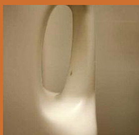
Untrimmed flashings on milk bottle handle
