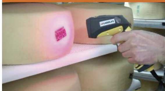
Capturing data from a caesin 2D Datamatrix code on cheese
