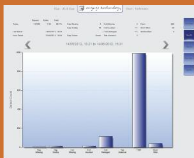
Milk bottle cap inspection – defect analysis
