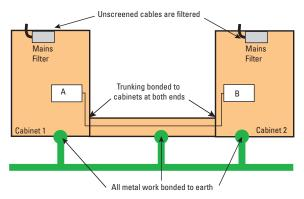
When installing screened cables the screen should not be used as a signal return path. For unscreened cables all signal and return cables should be twisted, i.e. Live & Neutral, 24v and 0v. It is important not to mix signal and return cables. When bonding other parts of machinery such as doors and lids etc. ensure that the earth straps have a large cross section. Braids or thick cables are normally used for these purposes. These should be kept as short as possible.
