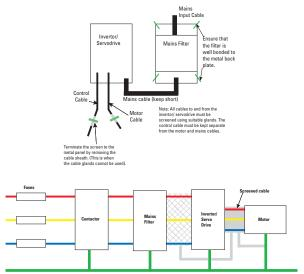
The above diagrams are used as a guideline only. It is recommended that you follow all of the manufacturers installation instructions where available. At frequencies above a few MHz, only an unbroken metal area or volume can achieve a reliable local RF reference, and only then for cables and electronics which remain within its boundaries. In the case of a metal sheet used as a local RF reference, the cables and electronics should remain close to its surface at all times.
