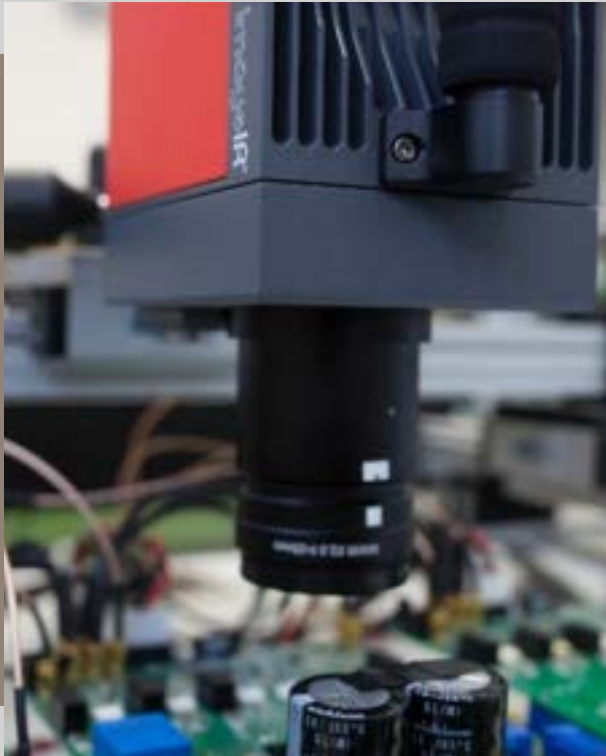
Fig. 2: Thermal setup with infrared camera and open semiconductor modules for thermal evaluation of the semiconductors during operation
