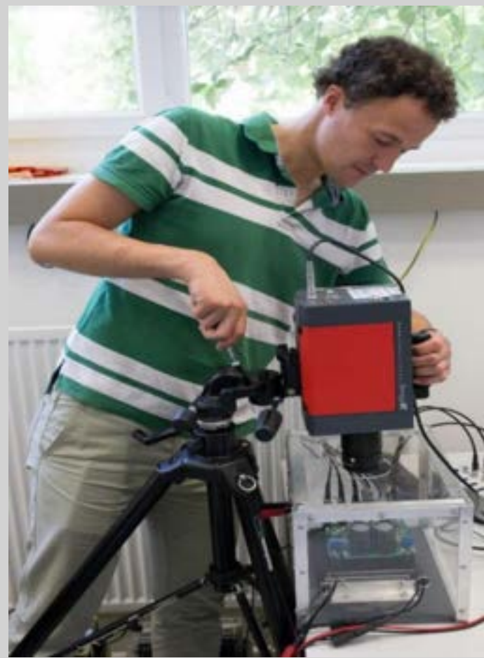
Fig. 3: Dr. Markus Andresen setting up the InfraTec infrared camera for tests to validate active thermal control
