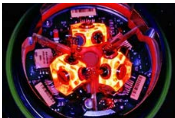
Figure 1. UV, EUV, and X-ray optics, such as the mirrors in this ring laser gyro, require supersmooth surfaces to avoid scattering that can impact performance and degrade the optics. (Rogoway)
