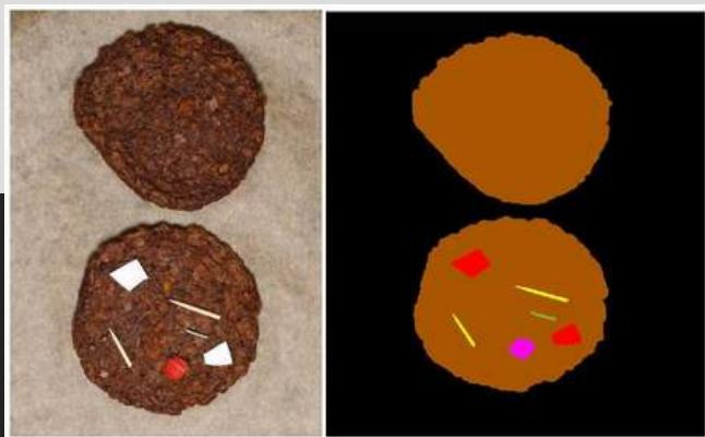
Fig 9. Veggie patties with contaminants: PS=red, PE=purple, wood=yellow), metal=green.
