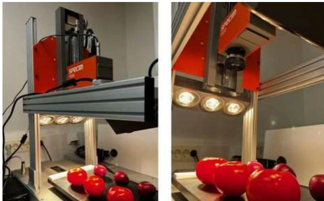
Fig 1: A sample of three plums and tomatoes placed on a lab scanner 40x20 and measured with a Specim FX10 camera for 20 days.
