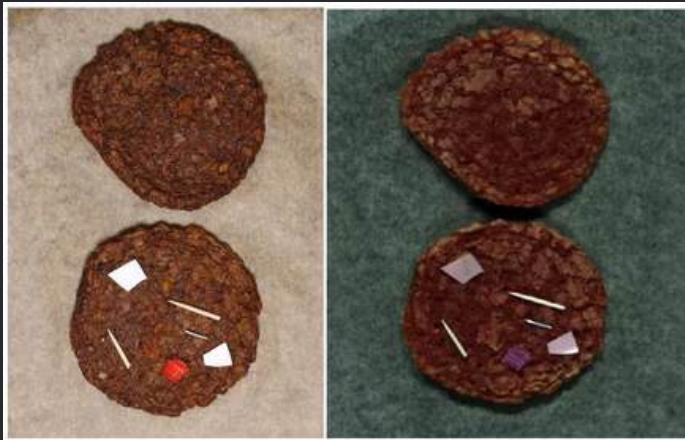
Fig 3. Veggie patties with contaminants. Photo (left) and hyperspectral false RGB image (right)
