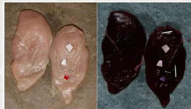
Fig 2. Chicken fillet with contaminants. Photos (left) and hyperspectral false RGB image (right).
