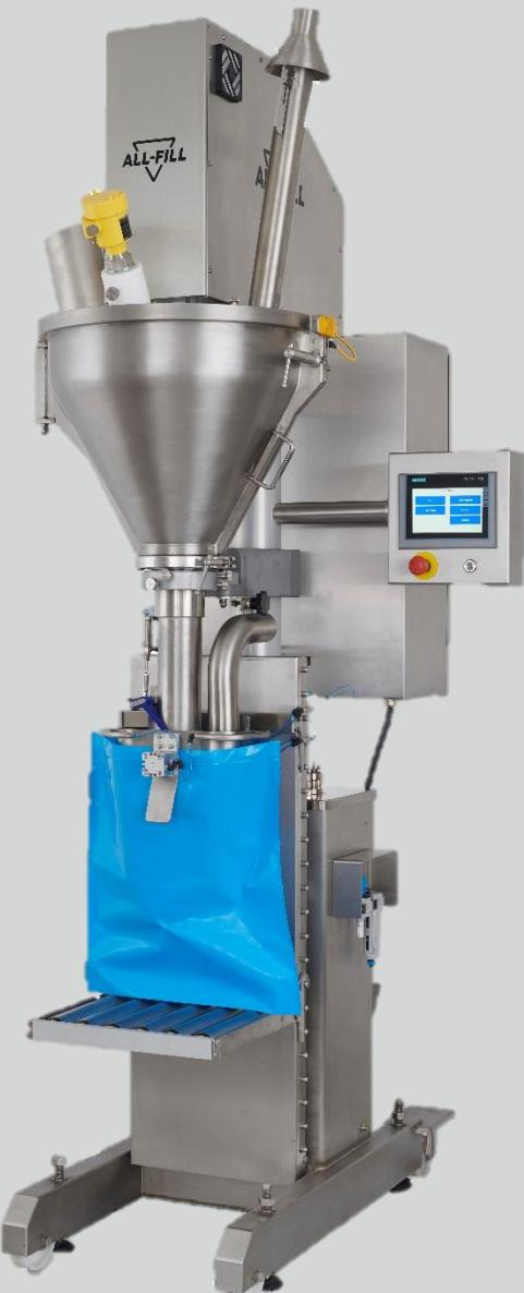
The All-Fill Series 10 Sack Filler has been specifically designed to accommodate a wide range of sack and bag sizes. The high-resolution digital strain-gauge load cell provides the signal for filling to stop, eliminating inaccuracies caused by products of inconsistent density. An electro-pneumatic clamp with easy-location presentation guides allows the operator to quickly place the sack/bag beneath the nozzle ready for filling.
