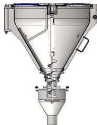
Straight auger with spinner plate ensures positive cut-off between fills. Funnel with optional dust extraction facility collects and guides product into containers.
