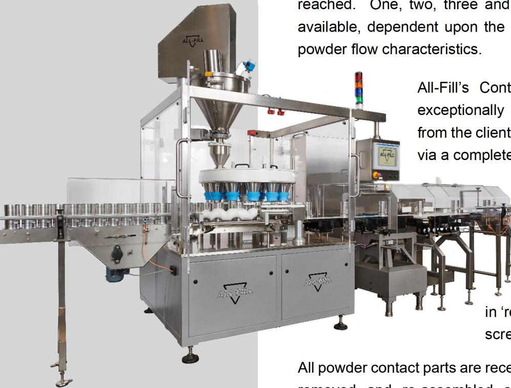
All-Fill's Continuous Motion Rotary systems fill exceptionally cleanly. The powder is progressed from the client's bulk feed system into the container via a completely sealed turret. The fillers can be offered with fully integrated check-weighing and reject systems, together with full feedback to the filling head. The fill weight performance of the filling machine can be displayed in 'real-time' graphical form on the touch-screen HMI.
