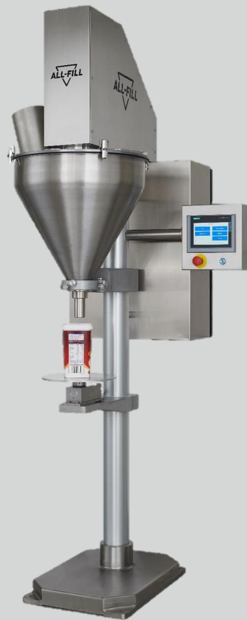
When filling gravimetrically, the All-Fill Series 10 fillers incorporate a weigh-cell or balance to provide the signal for the filling to stop, eliminating inaccuracies caused by products of inconsistent density.
