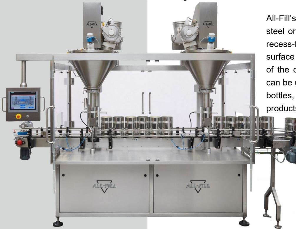
All-Fill's unique conveyor chain, stainless steel or plastic as appropriate, provides a recess-free wipe-clean stainless steel surface and affords access to the underside of the container for lifting. Neck locators can be utilised for centralising narrow-neck bottles, and vibration settling for granular products.
