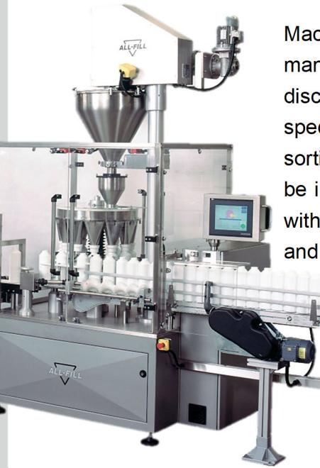
Machines are selected from specialist manufacturers following detailed discussions with the client to establish a specification. Functions such as container sorting/cleaning, capping and labelling can be incorporated into the filling line together with powder bulk feeding, metal detection and check-weighing systems.
