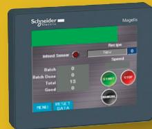
Fitted as standard with a touch screen HMI. Allowing you easy control over functions and the ability to save product settings.
