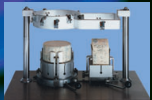
Horizontal and vertical portioning in one procedure.
