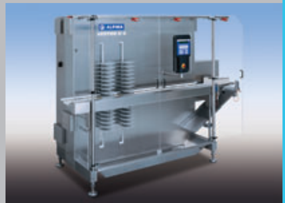
VESTOR II/S – vertical buffering for maximum space saving.
