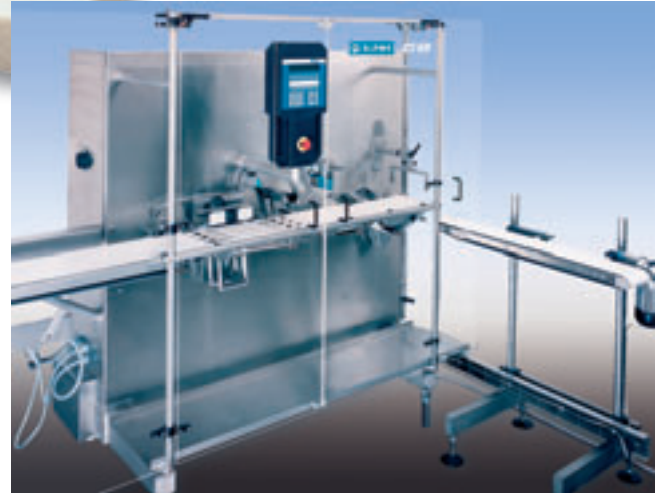
CUT 60 – cuts even extremely soft cheese into equal portions.
