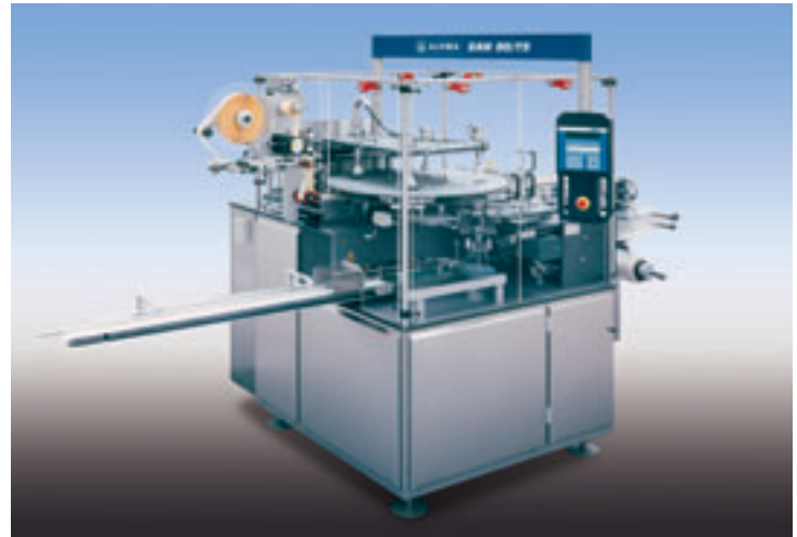
SAN 80/TS – high-performance packaging: 80 packs per minute.
