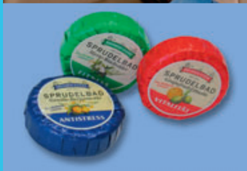
Pleat wrapping for round and spherical products.
