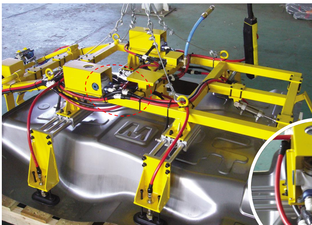
▲ Automobile Fuel Tank lifting (VTC3031 X 2 pcs)
