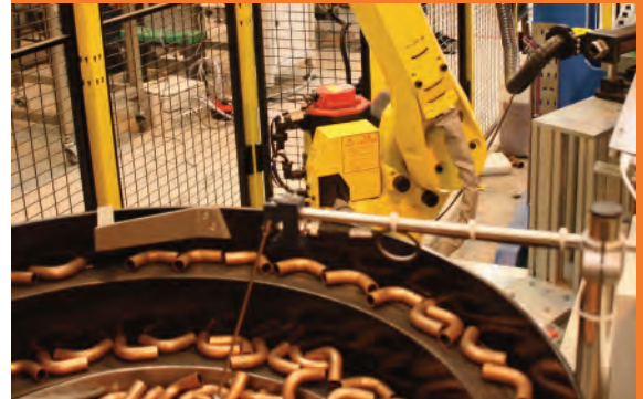
Plumbing parts on a Bowl Feeder below the vision guided robot
