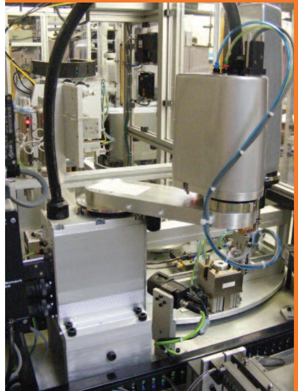
Automated spigot inspection system
