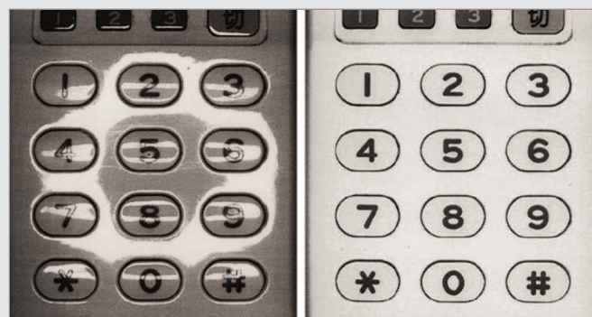
Polarising filter removes glare on keypad image (Courtesy Stemmer Imaging)
