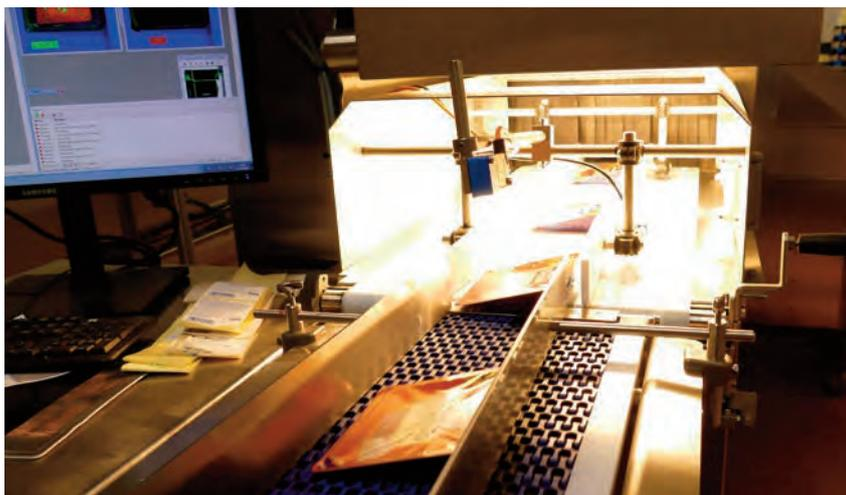
*Hyperspectral inspection of heat-sealed cheese packets*
