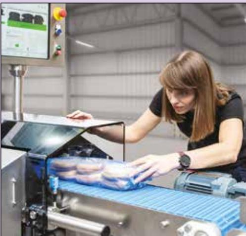
*IVS system for automated inspection of packaged breads*
