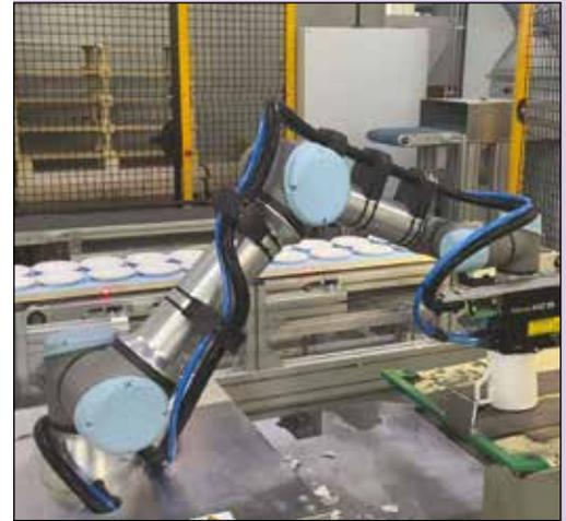
*Cobot-mounted 3D profile sensor for teacup pick & place*
