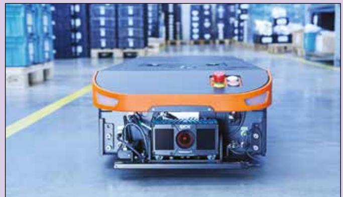
*Automated guided vehicle equipped with 3D time-of-flight camera (Courtesy Sick UK)*
