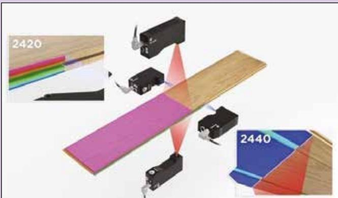
*Simultaneous wide field of view and high resolution 3D profile imaging of wood flooring panels (Courtesy Stemmer Imaging)*
