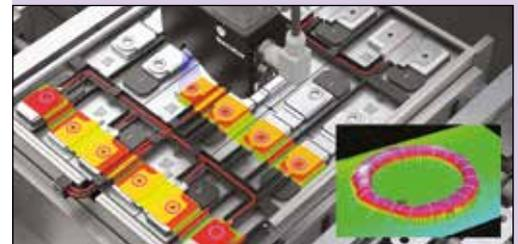
*Checking final weld quality on multiple battery cells*
